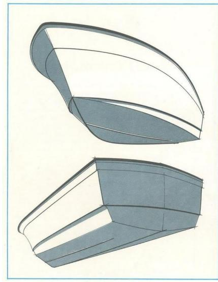
The 27' Commander hull starts with a sharply veed bow for a smooth entry through the water. The bottom sweeps gracefully into modified-vee planing surfaces. Longitudinal speed stabilizers provide superior control in turns and quartering seas. Additional stability is provided by the stepped chine, which also deflects spray. Note wide flare and marked flam in forward hullsides, which insure a dry ride.
