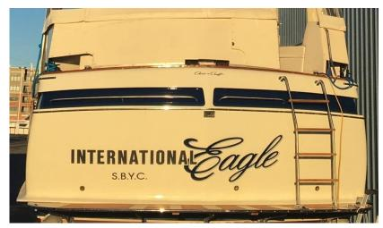
We rebuilt the transom boarding ladder treads and had a custom four-step swim ladder fabricated. The previous swim ladder was only two steps and when raised, didn't line up with the boarding ladder steps. This created a dangerous situation that could cause people to loose their footing on the unevenly spaced rungs. The new swim ladder perfectly lines up with the boarding ladder and essentially makes each step twice as deep when raised.
