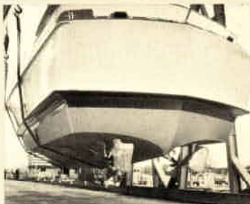
Hull of 38' Commander showing sharp vee entry, flared keel, speed stabilizers, hullside foil and vee transom.
