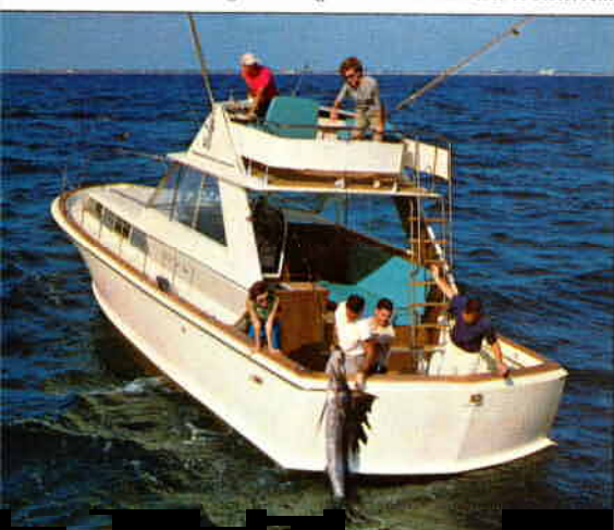
Sport Fisherman has uncluttered cockpit. No railings on coaming.
