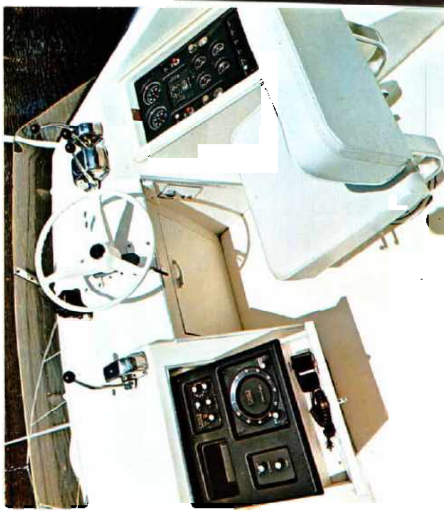
Command Bridge of a 35' Commander Sports Cruiser. The electronic bin, shown in the open position, houses the remote for the standard AM 100-watt radio-telephone and loud hailer; the optional 25-watt VHF-FM radio-telephone (upper right) and the optional depth sounder (lower right). Space is provided in the front of the bin for the microphone and the optional automatic pilot remote control assembly.
