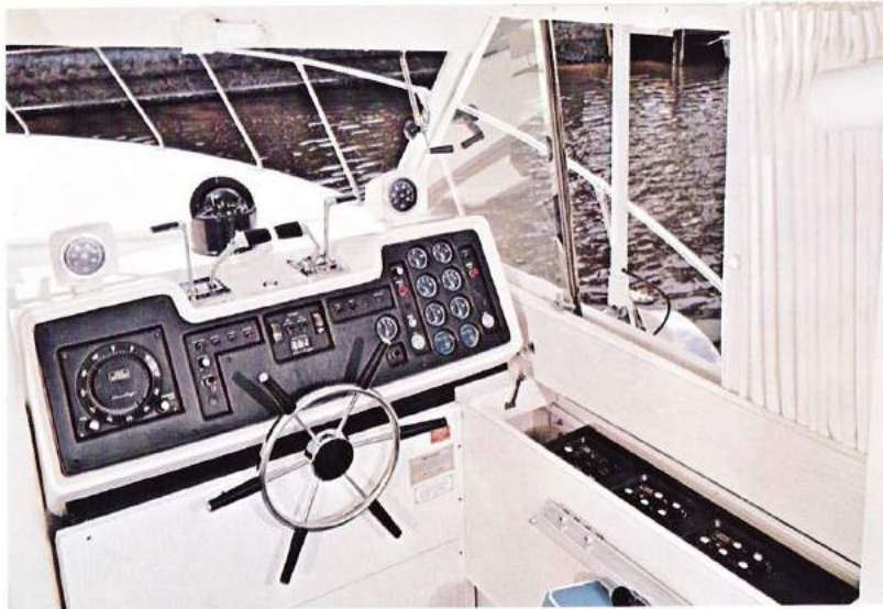
Lower helm station on a 35' Commander Sports Cruiser. Left of the wheel is the 60-foot-60-fathom depth sounder. In the locking cabinet outboard of the helmseat are the standard 100-watt AM radio-telephone and the electronic loud hailer plus the optional VHF/FM radio-telephone and automatic pilot.
