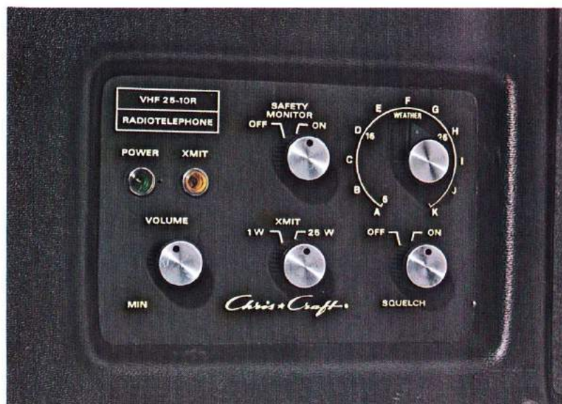
Control panels of all electronic components feature adjustable intensity back-lighting. This photograph shows the VHF/FM radio-telephone remote control panel illuminated at night.
