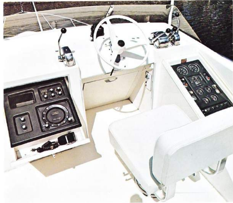
Command Bridge ® of a 35' Commander Sports Cruiser. The electronic bin, shown in the open position, houses the remote for the standard AM 100-watt radio-telephone and loud hailer, the optional 25-watt VHF/FM radio-telephone (upper right) and the optional depth sounder (lower right). Space is provided in the front of the bin for the microphone and the optional automatic pilot remote control assembly.
