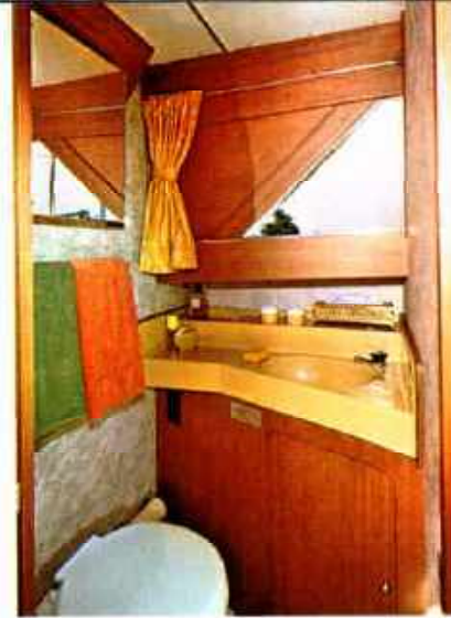
Lavatory has fiberglass sink and vanity.
