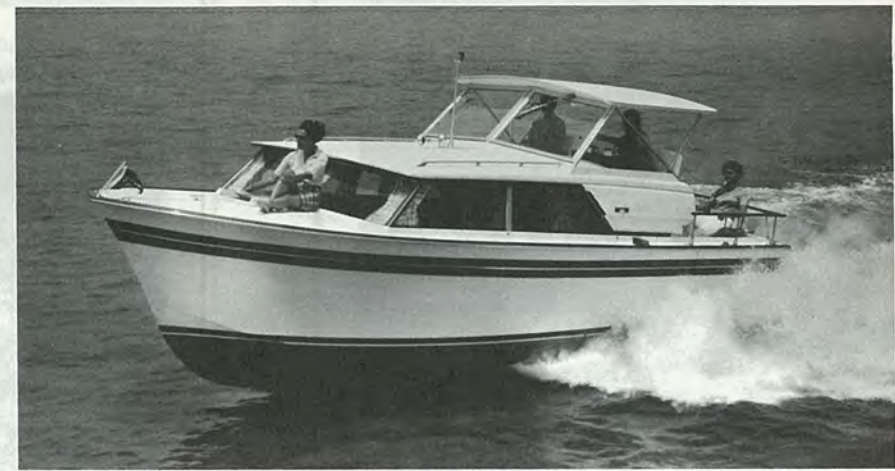
PLANKED PHILIPPINE MAHOGANY 30' CRUSADER. Accommodates six persons for cruising. V-berths forward have storage under. Convertible lounge and dinette areas; L-shaped galley, private lavatory, and plenty of storage. Twin 210-hp V8's; speeds to 34 mph. A hardtop is optional.
