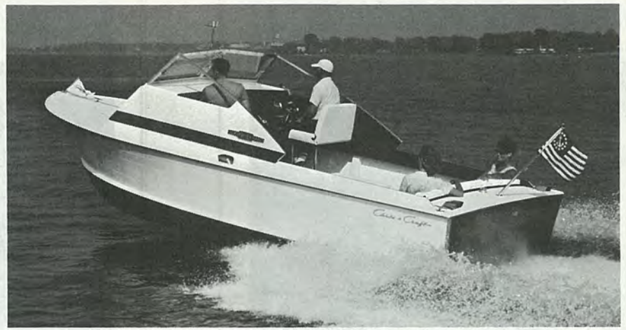
CARVEL SKIFF 25' CORINTHIAN SPORTSMAN. A versatile model that lets you make it what you will. Stern seat is standard. You can add helm and companion seats, mattresses, toilet, ventilating hatch, basic galley, hardtop, or folding top (all optional). 185 and 210-hp V8's; 32 mph.
