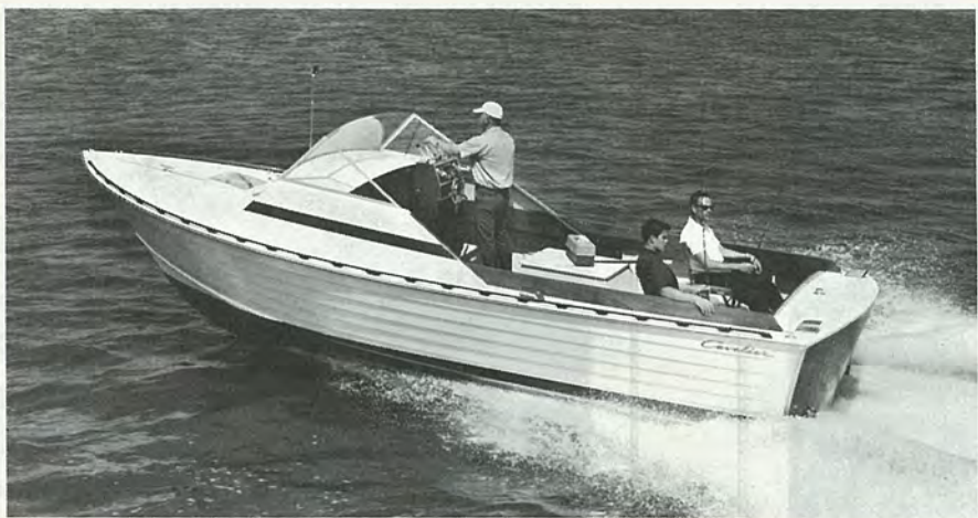
MARINE PLYWOOD CAVALIER 26' CUTLASS. Sportfishermen's favorite. Fast dry riding in offshore waters. Cuddy cabin has berth platforms, toilet, and locker. Galley unit, folding top, bow rails, helm and companion seats are optional extras. Single 210 or twin 185's; top speed is 36 mph.
