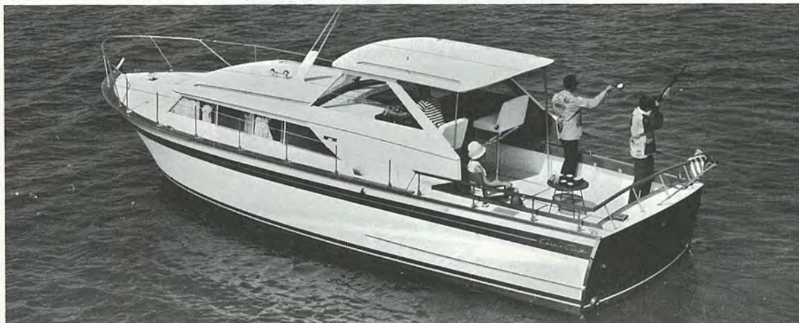
PLANKED PHILIPPINE MAHOGANY 36' CRUSADER. Cruises 6 persons with all the comforts of home. Private forward stateroom. Private lavatory (shower optional). Opposing lounge and dinette areas (both convertible). Twin 210-hp V8's; top speed is 32 mph. A fiberglass Command Bridge is optional.
