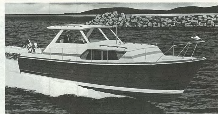
FULL LAPSTRAKE 31' CLIPPER CRUISER. Comfortable cruising for six. Private forward stateroom, roomy main cabin with convertible dinette and lounge, plentiful storage. Draperies are standard. Fully equipped galley. Options: hardtop; Command Bridge. Twin 210-hp V8's; speeds to 34 mph.
