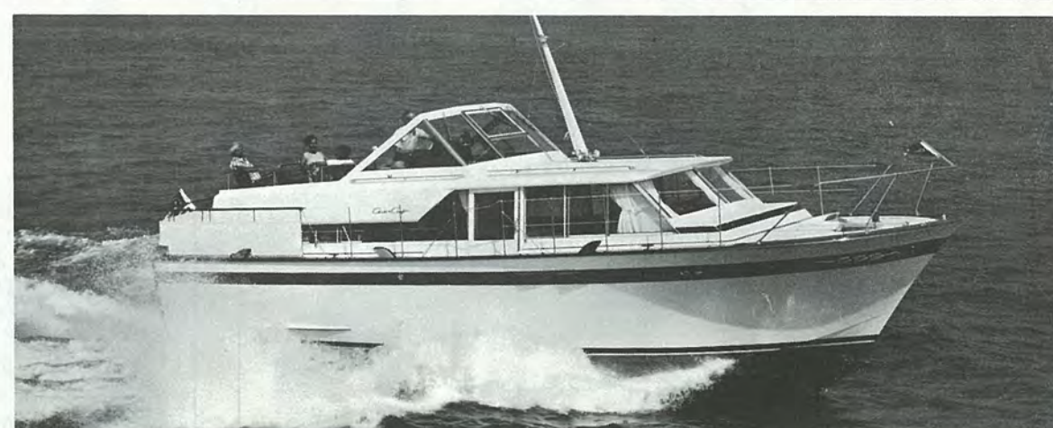
PLANKED PHILIPPINE MAHOGANY CHRIS-CRAFT 41' CONSTELLATION SALON . Sleek double-cabin model with extravagant space for cruising six or more. Shower standard in aft lavatory. Electric appliances in galley. Helm seat, compass standard. Twin 210's or 300's; 29 miles per hour.
