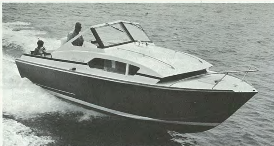
MARINE PLYWOOD CAVALIER 26' FUTURA. Advanced-design four-sleeper with V-berths, convertible dinette, galley, private lavatory. Vinyl-covered superstructure, decks, and cockpit floor. Fiberglass bottom covering optional. 185 or 210-hp V8 engine; hydraulic clutch standard. 30 mph.
