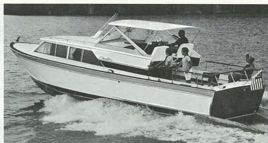
MARINE PLYWOOD CAVALIER 33' FUTURA. Deluxe six-sleeper with smooth hullsides. Private forward stateroom has large wardrobe, shipside shelves. Opposing lounge and dinette in main cabin. Twin 210-hp engines. Hardtop and Command Bridge optional.
