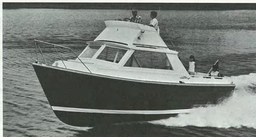
FULL LAPSTRAKE 28' CLIPPER SPORTSMAN. Can be semi-enclosed overnighter or fully enclosed cruiser. Helm seat standard. Options: Command Bridge, berths, toilet, galley, aft bulkhead with window and door, draperies. Single or twin 210's; speeds to 35 mph.
