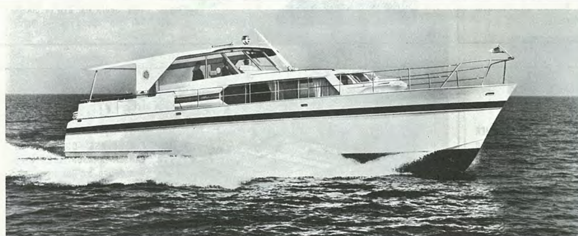
STEEL OR ALUMINUM ROAMER 57' MOTOR YACHT. Accommodations rival fine homes ashore, performance is unrivalled. Two staterooms aft with lavatory and shower, one stateroom forward with lavatory. Monel propellers and mufflers. 2" fiberglass engine room insulation. Diesels to 640 total hp. Cruise Control* standard.
