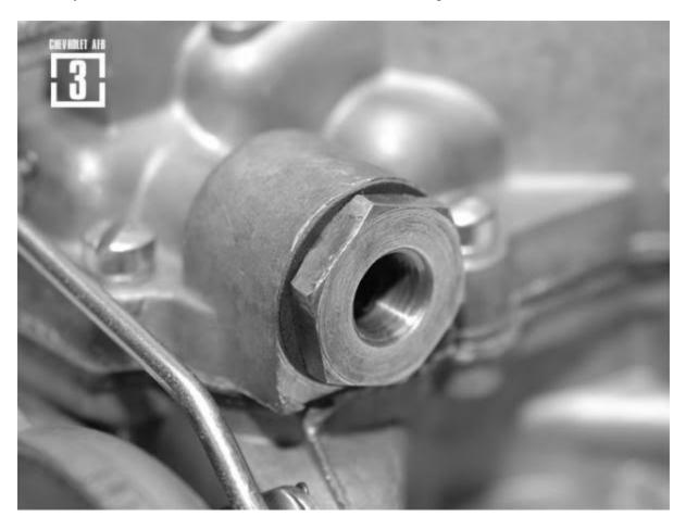
4 The choke unit on these earler versions is the same as on the WCFB's previously used. This style was replaced later by a more standard version, used by other brands.
