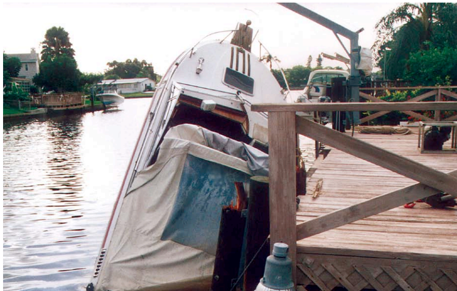
Rain or snow can make a boat too heavy for its lift.
