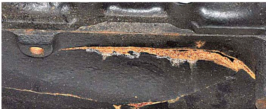
Water expands when it freezes and not properly winterizing your engine can lead to a cracked block, necessitating engine replacement.
