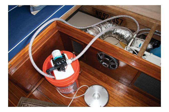
I began by gathering components in my shop. A 10-foot section of ½-inch water hose came first, then came several appropriately-sized nylon fittings (barbed and otherwise), an old, Pentair Shurflo Aqua King II water pump I had kicking around and, last but not least, a 5-gallon bucket. Before drilling my first hole, however, I did some preliminary research. Just for grins.
