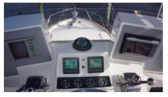
In 1994, a fly bridge with Bimini was added and later upgraded in 2010 with a new aluminum radar arch and console system. On the bridge, instrument clusters hold the needed GPS's, depth sounders, a PC navigation monitor and Simrad radar displays. One of the new additions is an instrument system, by CruzPro, that allows the digital display of all the pertinent engine, generator,
