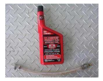
You need a foot and a half of 3/8 ID reinforced plastic hose from Lowes, a tire valve, three hose clamps, a tire pump or small 12 volt air compressor with a gage, and MMO.
