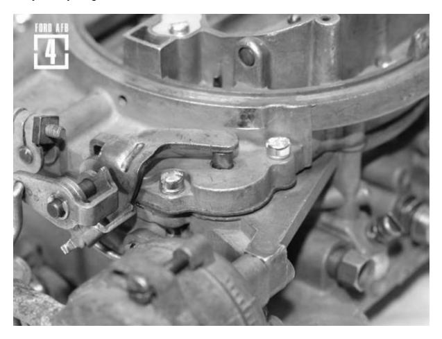
5. A water heated choke unit was used on the Lincoln line up. A Ford only feature and a sign of the things to come. Different and innovative.
