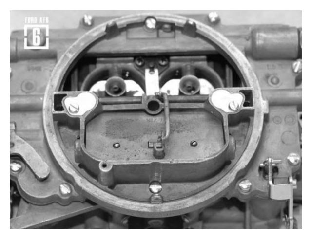
7 Picture showing the placement for Fords own ID number. The four digit stamp was placed on the LH, at front of the baseplate as usual. As always ending with an S or SA.
