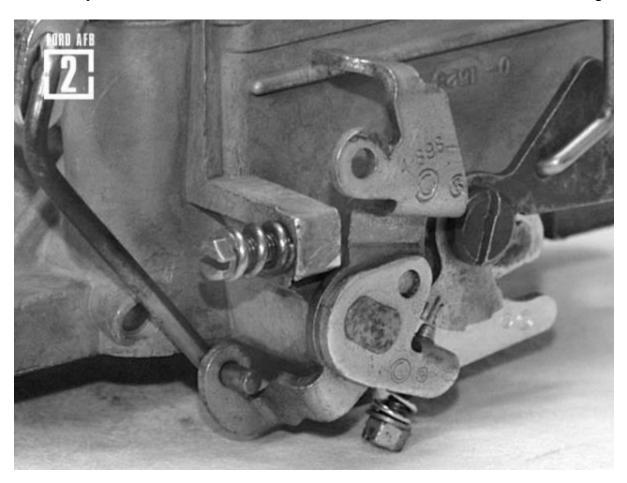
3 The fuel inlet is placed on the LH side. We can also spot a glimpse of the overhead choke type, more common on the later model AVS type carbs.
