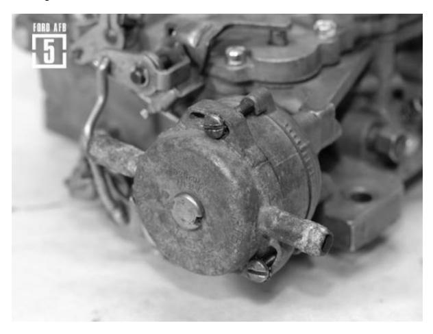
Easy to spot from the outside. The big air horn,  $5\ 1/8$ " in diameter, was used to faciliate the use of Fords own air cleaner units.
