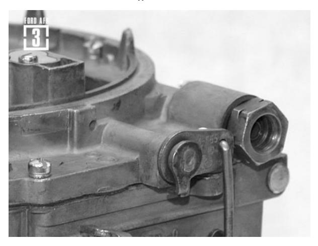
4. Lincoln used a integrated type of dash pot. Basically a accelerator pump-stem which was dampened by the gasoline in the float bowl
