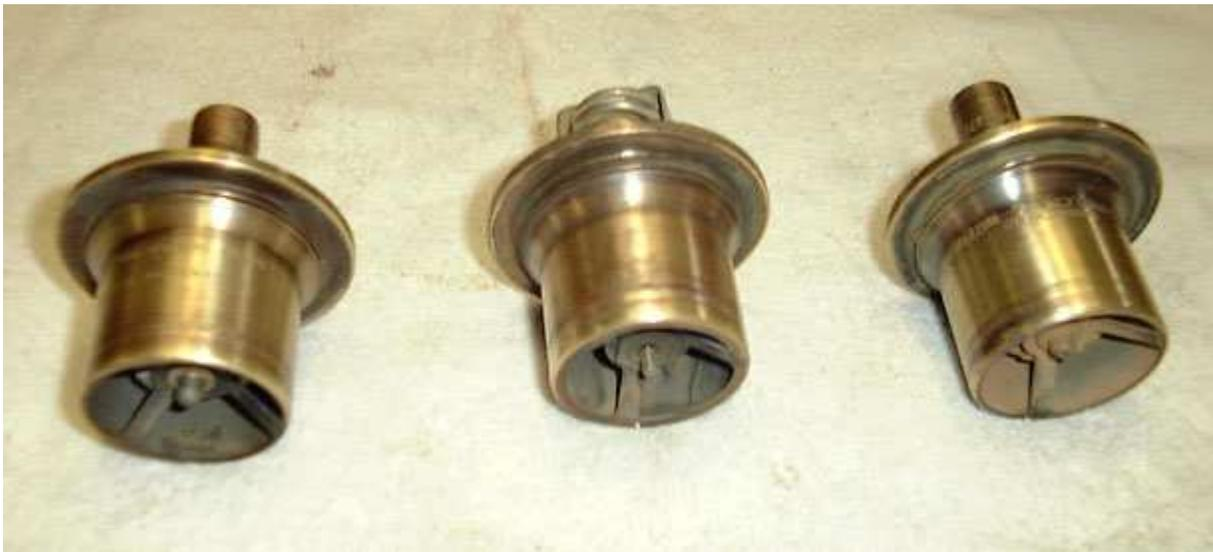
T1 & T2 - These 2 shots show my three spare stats. The one in the middle is an "oddball" that I bought from a parts bin. I believe it's a Chrysler inboard engine stat from the 80's. The physical dimensions are the same. It's marked "ST 358", & 140 is stamped under the 358 number. The outside 2 stats are the originals in my 427's. Rostra Vernatherm manufactures them, and the number is "Vernatherm Valve VD111458B". On the nose is stamped 130 C 89 4 on one stat,
