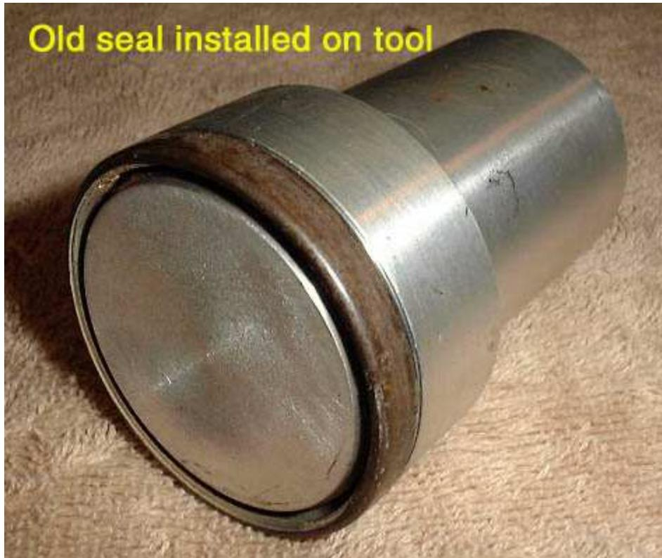
T5 - This shot shows one of my old seals mounted on the nose of my tool, ready to be tapped into it's bore in the circulating water pump housing.
