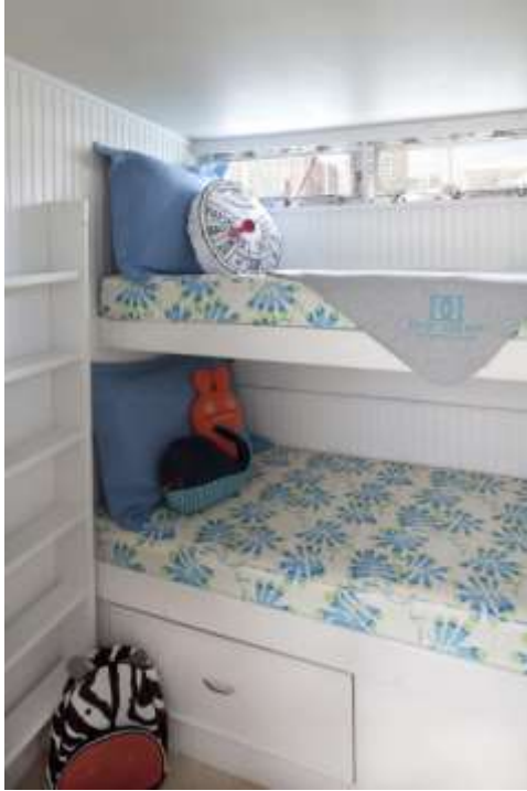
Walls are clad in marine grade vinyl or teak bead board, lacquered in marine grade finish.
