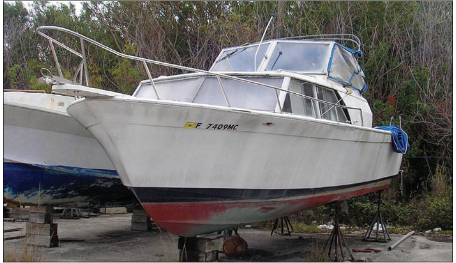
Above —The Commander as found in Florida. The boat was in sound structural condition, had the advantage of a simple single-engine configuration, and a relatively efficient, dry-running hullform. Below —Much of the wood interior had been ruined by rodents and water intrusion.
