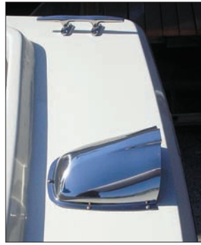
Above —The severely corroded original chromed vent covers were replaced with off-the-shelf stainless models.
