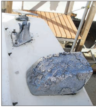
Above —The severely corroded original chromed vent covers were replaced with off-the-shelf stainless models.
