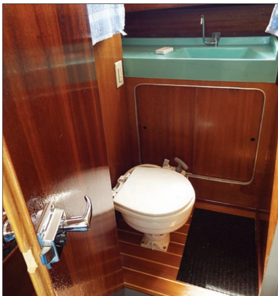
Left —The molded fiberglass lavatory sink in the head compartment was one of the few salvageable elements from the original interior. The mahogany bulkheads were also saved and refinished. Right —The new galley includes new gas cooktop, shelves, racks, lighting, a black composite sink (covered with a cutting board), a new refrigerator, and a veneered counter with inlaid ceramic tiles.
