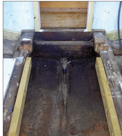
Left —The aging gas engine in the abandoned boat was spent. Right —The oily bilge under the engine had to be thoroughly cleaned, the high engine beds cut away, and new lower beds lagged and epoxied to the original fiberglass stringers to accommodate the new engine.
