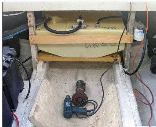
Left —A new 74-gal (280-l) plastic fuel tank replaced the corroded original steel cylindrical model, adding 20 gal (70 l) to the fuel capacity and shifting its center of gravity several feet forward. Right —One of the toughest, most time-consuming jobs was removing the old Cutless bearing, which had seized in the strut. It had to be largely cut away, with great care not to damage the strut.
