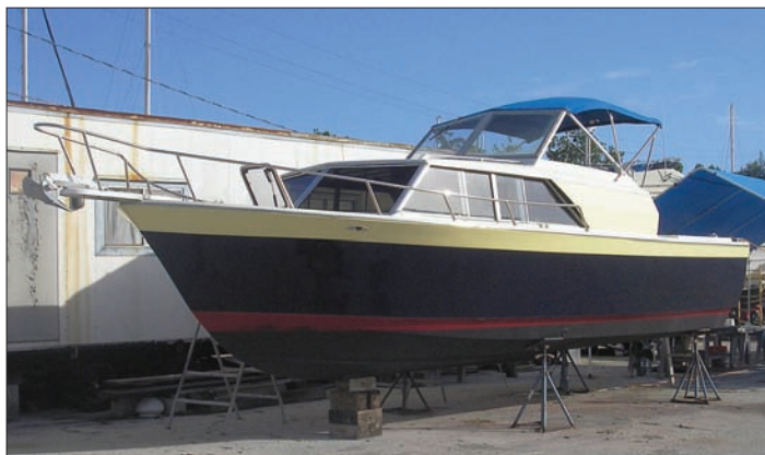
Left —The repaired and faired topsides were primed with a high-build primer followed by Awlgrip 545 gray epoxy. Right —The top-side finish paint is Nauticoat. Following that, the stainless rubrails, forward rails and pulpit, and aluminum trim were reinstalled.
