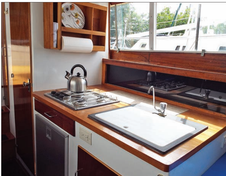
Left —The molded fiberglass lavatory sink in the head compartment was one of the few salvageable elements from the original interior. The mahogany bulkheads were also saved and refinished. Right —The new galley includes new gas cooktop, shelves, racks, lighting, a black composite sink (covered with a cutting board), a new refrigerator, and a veneered counter with inlaid ceramic tiles.
