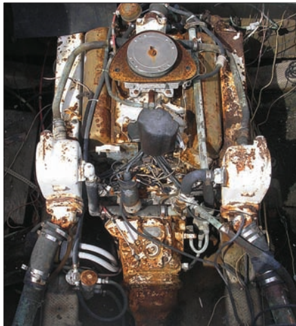
Left —The aging gas engine in the abandoned boat was spent. Right —The oily bilge under the engine had to be thoroughly cleaned, the high engine beds cut away, and new lower beds lagged and epoxied to the original fiberglass stringers to accommodate the new engine.
