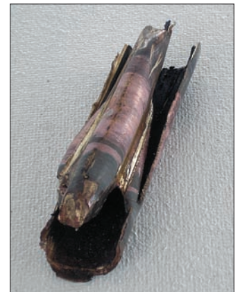
Left —A new 74-gal (280-l) plastic fuel tank replaced the corroded original steel cylindrical model, adding 20 gal (70 l) to the fuel capacity and shifting its center of gravity several feet forward. Right —One of the toughest, most time-consuming jobs was removing the old Cutless bearing, which had seized in the strut. It had to be largely cut away, with great care not to damage the strut.
