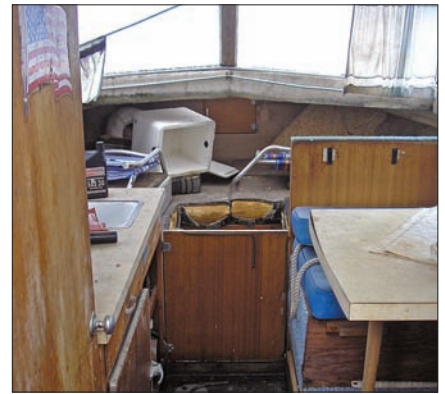
Above —The Commander as found in Florida. The boat was in sound structural condition, had the advantage of a simple single-engine configuration, and a relatively efficient, dry-running hullform. Below —Much of the wood interior had been ruined by rodents and water intrusion.
