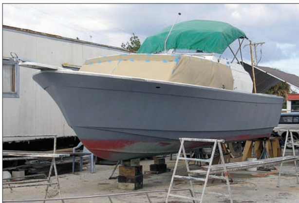
Left —The repaired and faired topsides were primed with a high-build primer followed by Awlgrip 545 gray epoxy. Right —The top-side finish paint is Nauticoat. Following that, the stainless rubrails, forward rails and pulpit, and aluminum trim were reinstalled.
