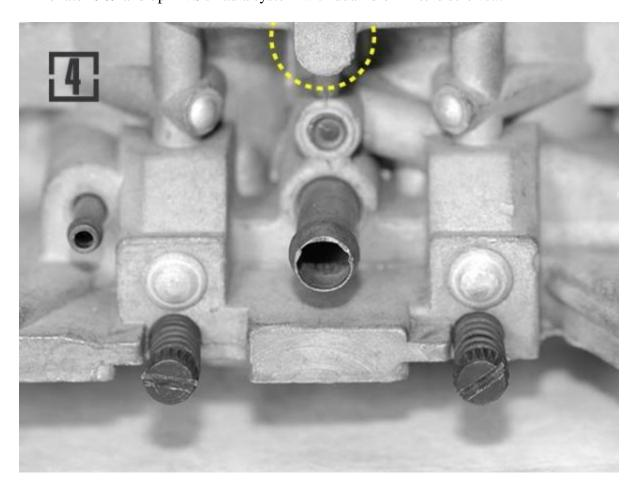
5 ...as opposed to the earlier versions, that uses one mixture screw. Works like this. To enrich mixture, turn clockwise. To lean out mixure, turn ccw. Take caution, it has LH threads! A modern name would be "reverse idle system".
