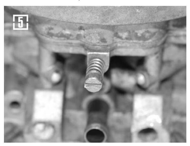
6 Here is the explanation why it is named AVS, air valve spring. The valve is governed by the spring, that is adjustable. This feature was carried over to the Thermoquad.
