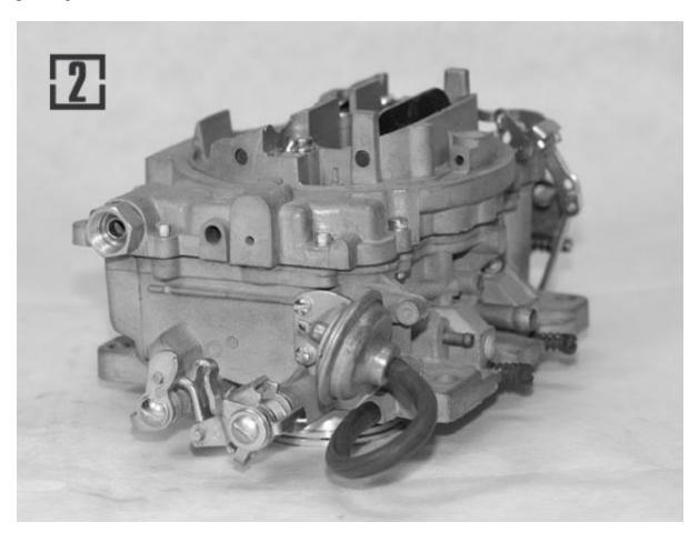
3 The application and date code was stamped in the same location as the AFB. An ID tag was also used for identification.
