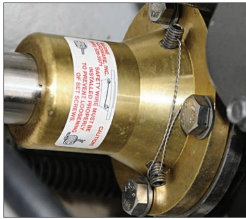
Far left —Grease on this coupling and key was applied to ease installation but will actually prevent full engagement between the shaft and coupling, as it cannot be compressed in the confined coupling bores. Shafts, keys, and couplings may be lightly oiled to prevent binding and ease installation. Left —This brass taper coupling relies on set screws to secure the shaft end nut. Note that the seizing wire is correctly tensioned to rotate the screws clockwise.
