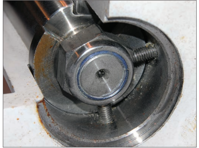
Left —Tapered couplings offer several advantages over straight and split models. The interface between the taper shaft and the bore makes for an exceptionally tight fit. In some cases where locking nuts have loosened, the shaft and coupling must still be separated with a hydraulic puller. Right —This tapered coupling has the added security of set screws to retain the locking nut.
