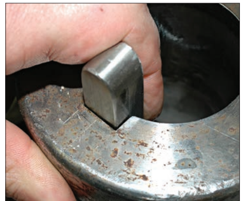
Left —A ramped and radiused keyway is more resistant to stress-induced fractures, while the knurling improves the interference fit on this small sail auxiliary straight-bore coupling. Right —Keys should fit snugly into a keyway and, when lightly oiled, should slide and be easily removed. Unlike this one, they should not rock or clack when moved from side to side.
