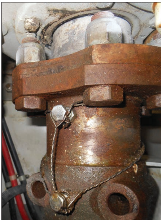
Left —Set screw tips should be either cupped or pointed, and hardened. Ordinary stainless steel fasteners, shown here, should not take the place of purpose-built screws. On the plus side, these set screws are secured with locking nuts and seizing wire. Above —Scallops cut into this shaft indicate that it's designed for use with a split coupling. Pinch bolts interface with the machined dimples to improve shaft-to-coupling engagement.
